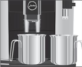
When the JURA is switched off, the system is automatically rinsed if a speciality coffee has been prepared.
